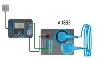
Figure 5.1: Application example using MI 3365 and A 1832 (Continuity of PE conductor)
