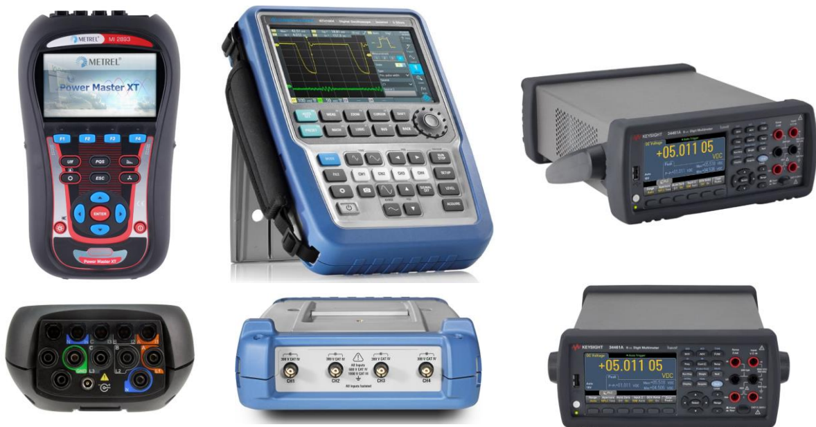
Figure 96_Typical devices with floating inputs
