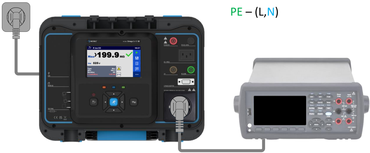
Figure 102_Insulation resistance Class I
