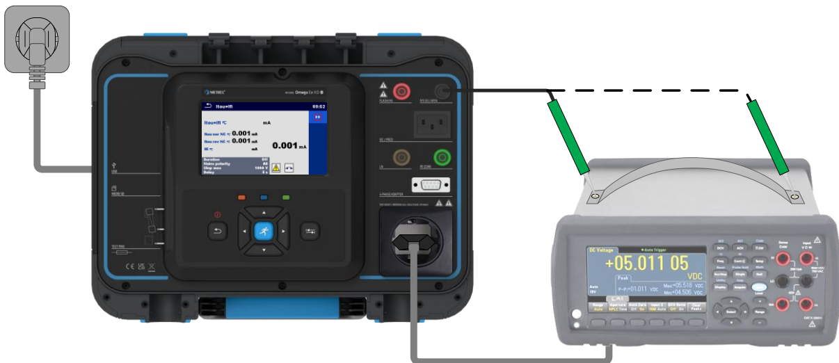
Figure 108_Touch leakage current (Class II)
