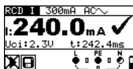
Figure 5.20: Trip-out current measurement result example
