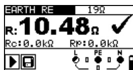
Figure 5.35: Example of earth resistance measurement result
