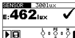
Figure 5.65: Example of illumination measurement result
