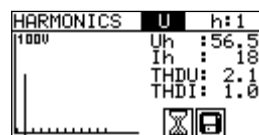
Figure 5.49: Examples of Harmonics measurement results
