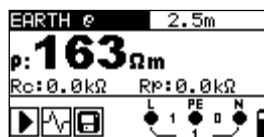
Figure 5.42: Example of specific earth resistance measurement result
