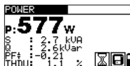
Figure 5.47: Power measurement results
