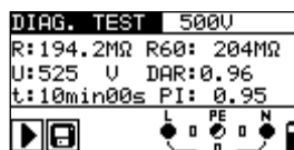
Figure 5.10: Example of PI and DAR diagnostic test results
