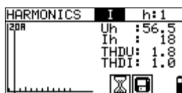
Figure 5.49: Examples of Harmonics measurement results
