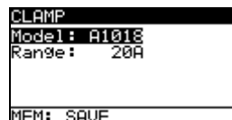
Figure 4.13: Configuration of current clamp measuring input
