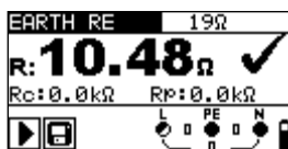
Figure 5.38: Example of earth resistance measurement result
