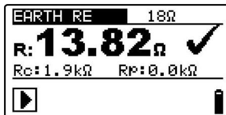
Figure 5.4: Example of earth resistance measurement result
