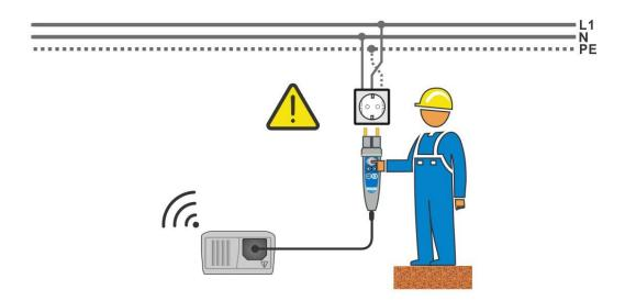
Figure E.4: Reversed L and PE conductors (application of plug commander)
