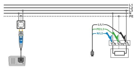
Figure 5.24: Connection of plug commander and 3-wire test lead
