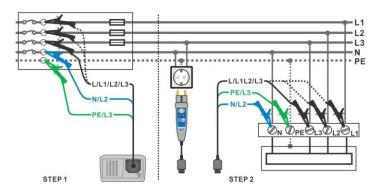
Figure 5.30: Phase-neutral or phase-phase voltage drop measurement – connection of plug commander and 3-wire test lead
