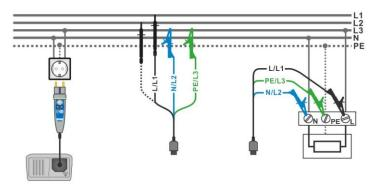
Figure 5.28: Phase-neutral or phase-phase line impedance measurement – connection of plug commander and 3-wire test lead
