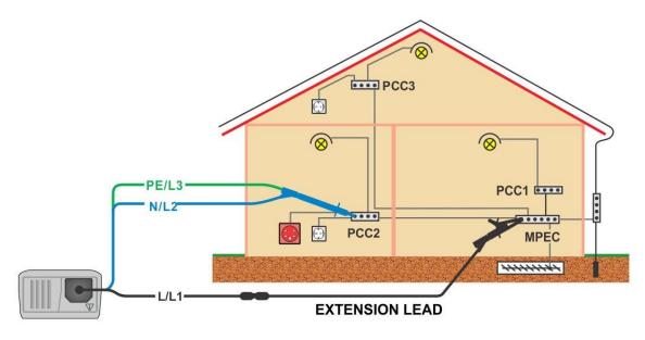
Figure 5.9: Connection of 3-wire test lead plus optional extension lead
