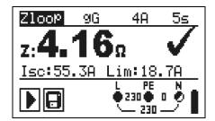
Figure 5.25: Examples of loop impedance measurement result
