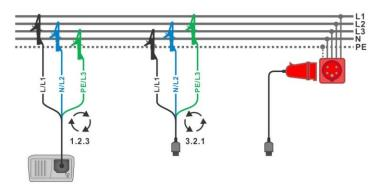
Figure 5.2: Connection of 3-wire test lead and optional adapter in three-phase system
