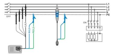
Figure 5.6: Connections for insulation measurement
