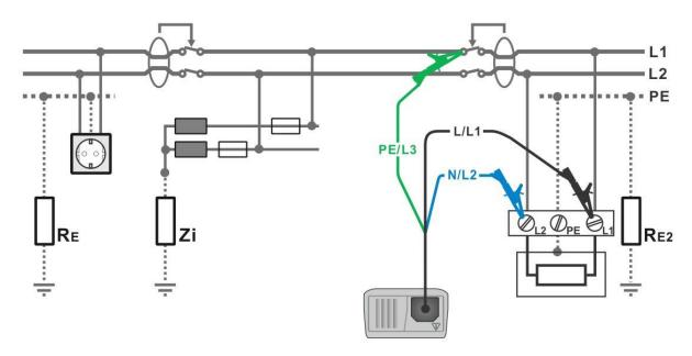
Figure D.3: RCD testing in IT system with bypassing RC
