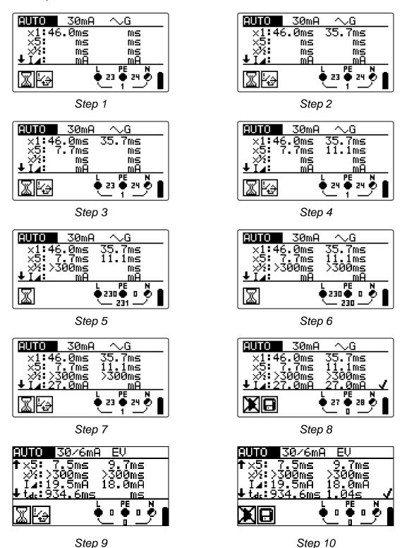
Figure 5.21: Individual steps in RCD autotest
