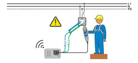
Figure E.5: Reversed L and PE conductors (application of tip commander)
