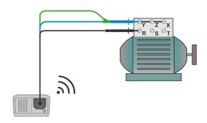
Figure 5.11: 3-wire test lead application
