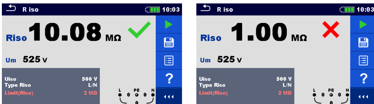
Figure 7.9: Examples of Insulation resistance measurement result
