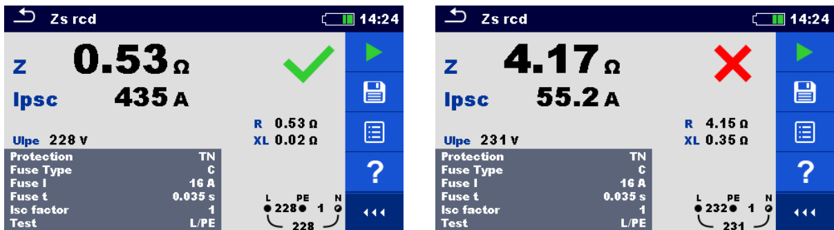
Figure 7.38: Examples of Zs rcd measurement result
