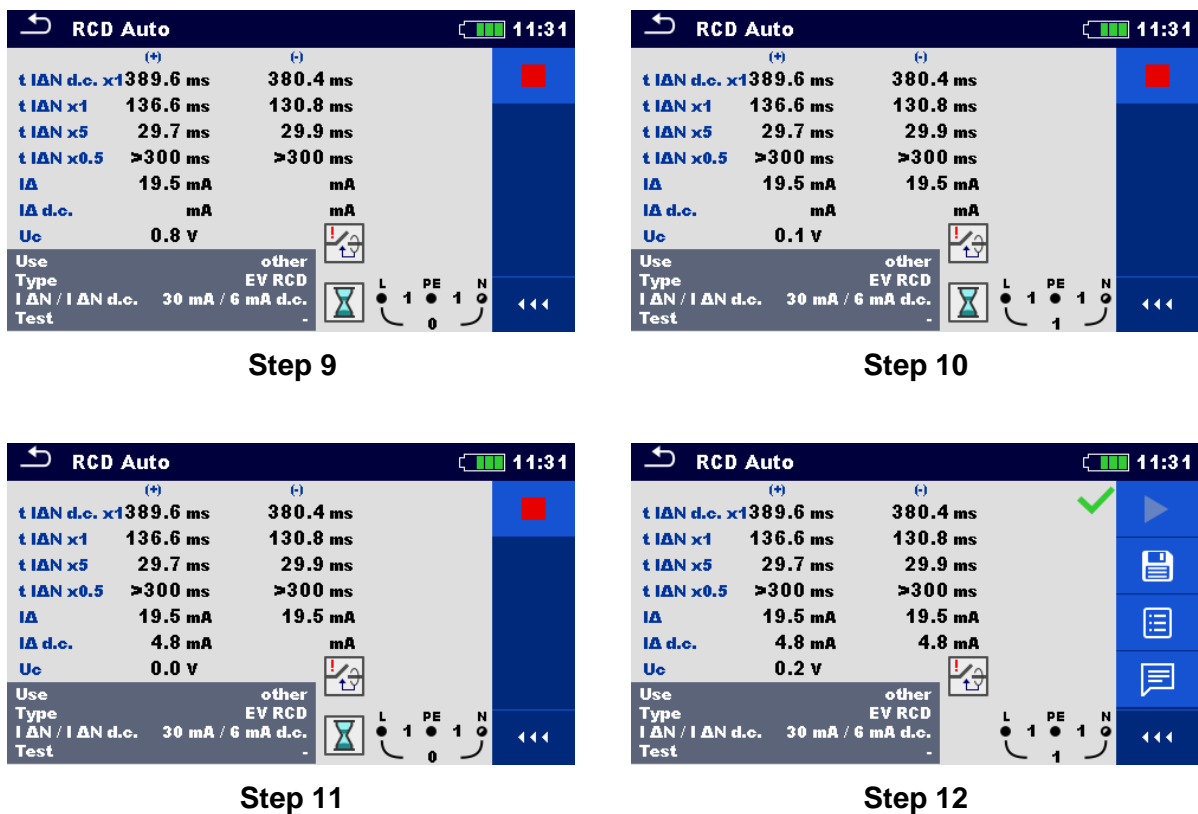
Figure 7.32: Example of individual steps in RCD Auto test, example on testing EV RCD
