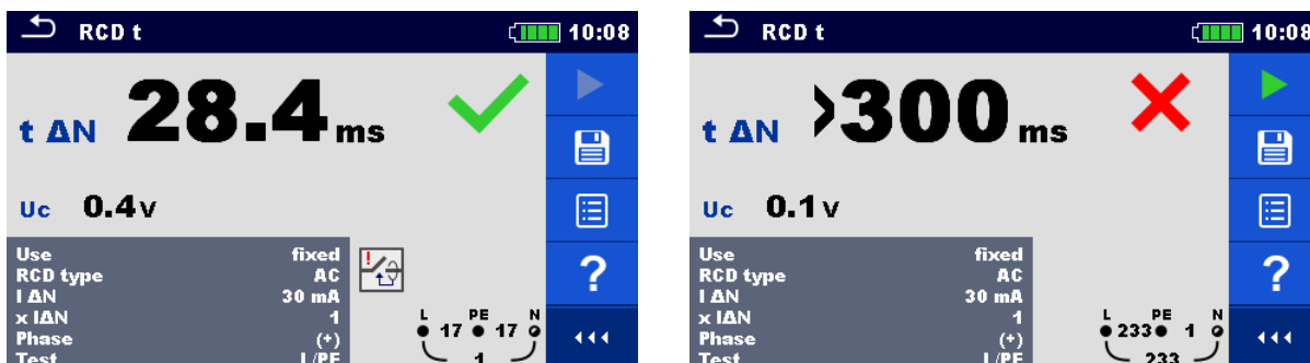
Figure 7.30: Examples of Trip-out time measurement result
