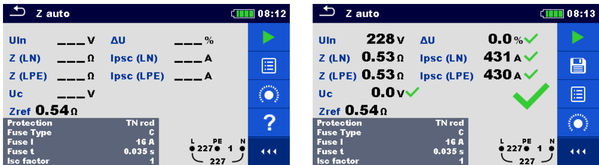
Figure 7.107: Example of Z auto measurement results
