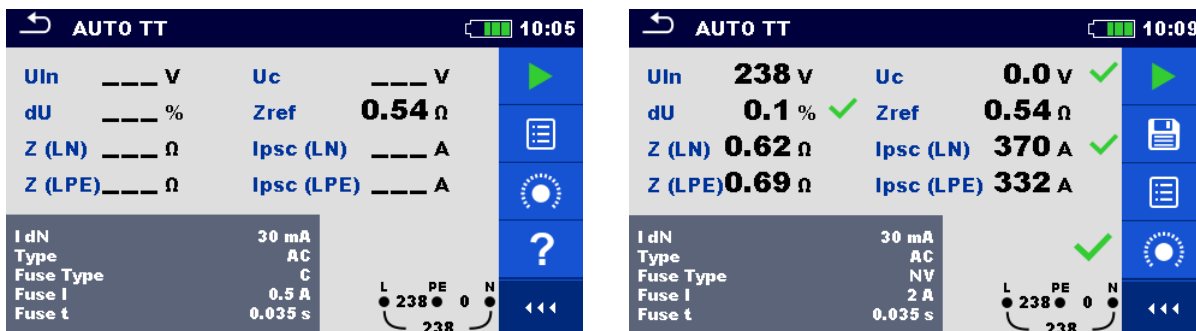
Figure 7.95: Examples of AUTO TT measurement results
