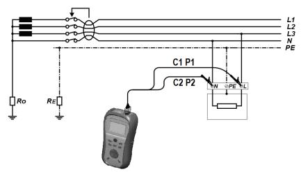
Figure 6.9: Voltage TRMS connection
