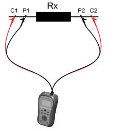
Figure 6.3 Resistance measurement connection
