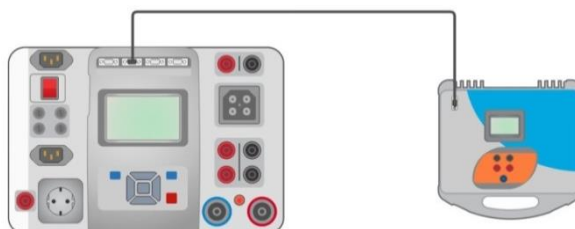
Figure 8.2: Connection of the Euro Z 290 A adapter A 1143
