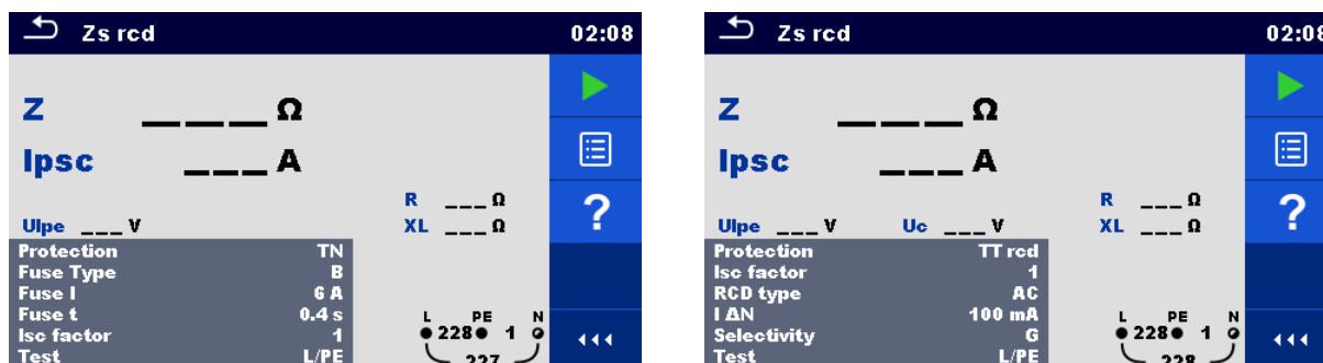
Figure 6.72: Fault loop impedance and prospective fault current Zs rcd test menu
