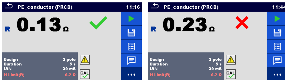
Figure 6.120: Examples of PE conductor (PRCD) results
