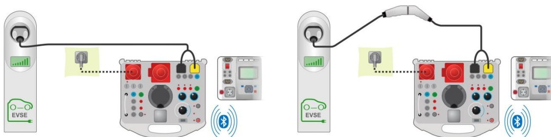
Figure 6.104: Diagnostic test - EV simulator and Errors sub-tests - connection to EVSE
