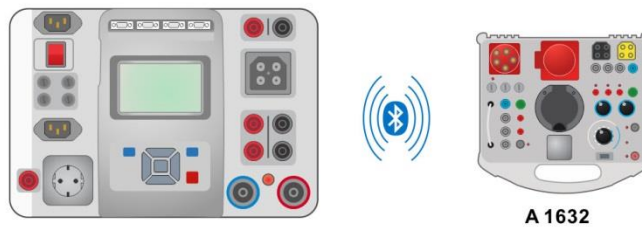
Figure 8.4: Connection of the eMobility Analyser (A 1632)
