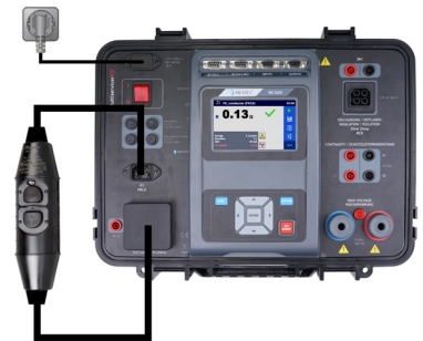
The PE conductor test and polarity test.
