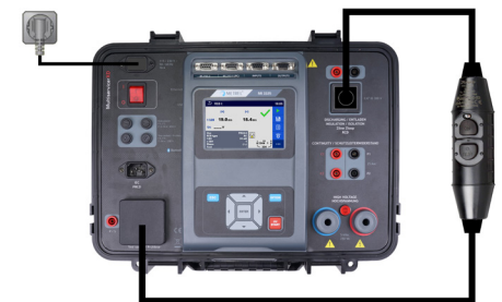
The measurements of trip out time and trip out current.
