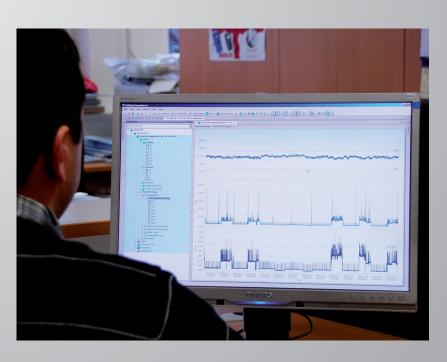
PowerView3 software is a powerful platform for downloading, analysing recorded data and creation of power quality test reports. PC Software contains a package of functionalities needed for profound evaluation of power quality phenomena, data comparison and creation of complex test reports. It works in conjunction with Metrel new generation power quality analysers. For the instruments equipped with GPRS functionality PowerView3 enables remote control of the instrument as well.
