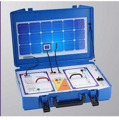
Demonstration board MI 3088 simulates typical photovoltaic (PV) system with one PV module and DC/AC inverter. It represents a typical installation that consist of PV string, DC switch box, DC/AC inverter and one phase connection to the power grid. It is intended for use preferably by sales personnel for demonstration of the measuring methods and procedures on DC and partially on AC side of a PV system.
