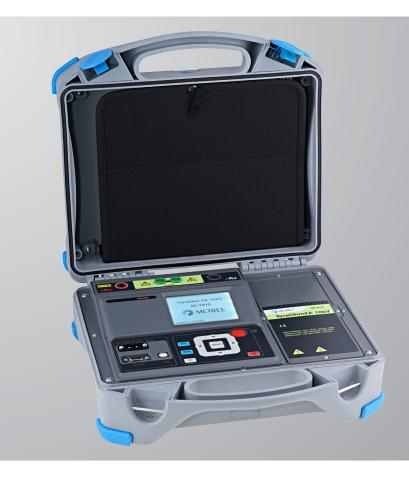
MI 3210 TeraOhm XA 10 kV is a portable, battery or mains powered test instrument with excellent IP protection (IP65), intended for diagnosing of Insulation Resistance by using high DC test voltages of up to 10 kV. Because of its robustness (CAT IV protection) and high immunity to radiated RF fields it is best suited for industrial environment
