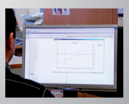
The HVLink PRO software works in conjunction with Metrel newest HV insulation testers, Step Contact Voltage Measuring System and MicroOhms. The software automatically recognizes connected instrument and allows the customer to download test results saved on the instrument, review the results, rename and relocate data if needed and print test reports.
