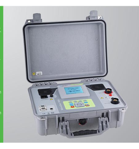
portable low resistance ohmmeter used to measure low contact resistances of circuit breakers, switches and busbar joints using test current from 100 mA to 100 A. Used 4-lead Kelvin testing method ensures very high accuracy of results (0.25%) due to elimination of test leads resistance. The instrument can be powered from both mains supply and internal battery. PC SW HVLink PRO supplied as a standard accessory enables downloading, analysis and export of test results and printing of test reports.
