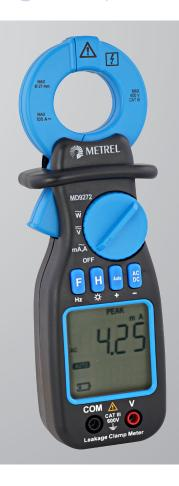
The MD 9272 is a unique earth leakage clamp meter. It not just has the ability to accurately read the TRMS AC leakage current of a system, it can also detect losses in the system and suggest possible reasons for the loss. The voltage, power, harmonic, power factor (PF), total harmonic distortion (THD) and crest factor measurements make this instrument suitable for any electrician and engineer
