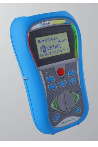
MI 3242 MicroOhm 2 A is a portable low resistance ohmmeter used to measure low resistances of switches, relays, connectors, bus bars, power distribution cable joints, motor & generator winding, power transformers, power inductors, rail track joints, wire and cable resistance, welding joints for industrial application, etc., with test current up to 2 A.
