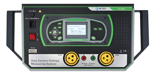
The MI 3295 Step/Contact Voltage Measuring System is a voltage measuring system intended for testing and verification of protective earthing of power stations, substations and other power systems. It is one of the smallest solutions on the market but cleverly designed to balance between safety, powerful generator (up to 55 A) and special technology
