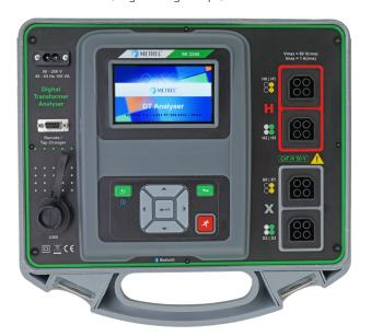
and bad contacts. The MI 3280 Digital Transformer Analyser is powerful single and three phases solution for automatic testing of any vector group of LV and MV transformers. Beside transformer turn ratio test, MI 3280 allows also measurement of transformer winding resistance, which could be periodically performed to inspect the transformer condition.
