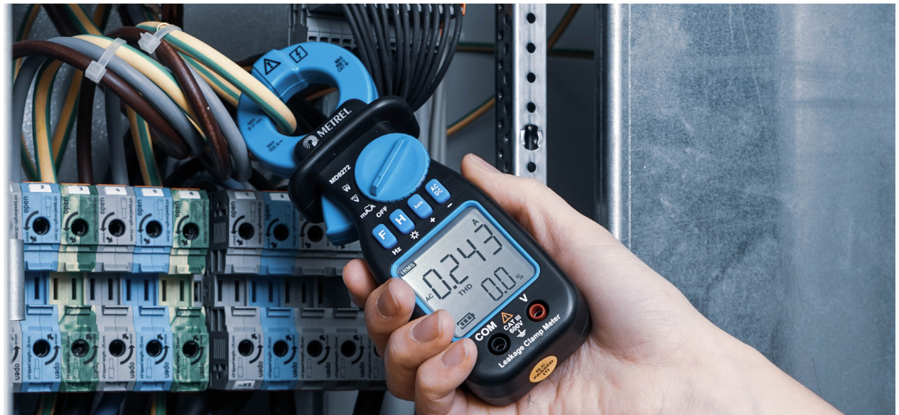
Measuring leakage current at the edge of an isolated island.
