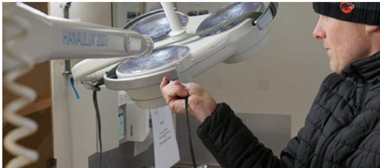
Measuring continuity of protective earth on mobile medical equipment is no different from fixed versions.
