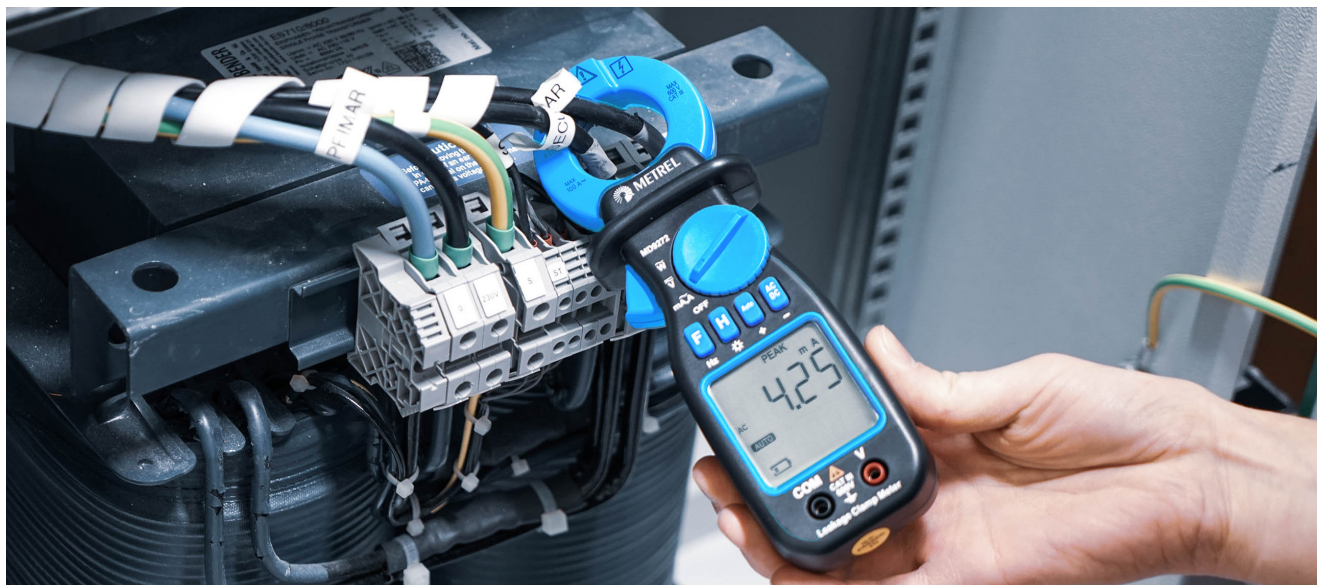
Leakage current measurement at RCDs is one of diagnostic tests.
