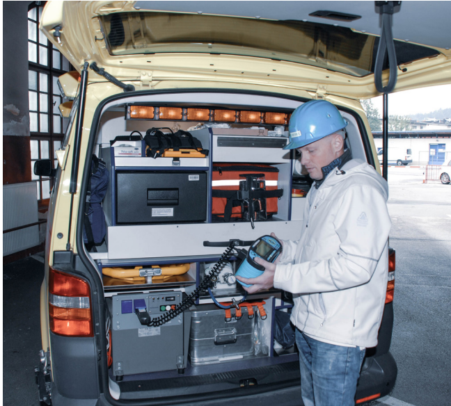
Testing the control panel of secondary power source in an ambulance.
