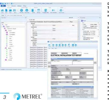
Depending on the instrument model or type the user can create AU-TOSEQUENCEs, custom tests or single tests. They can be integrated into the custom created test structures and then uploaded into the measurement instrument
