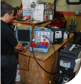
The A 1422 Multifunctional test adapter has all functionalities as its predecessor A 1322 plus complete support for testing of Arc Welding Equipment. This makes it a perfect test and troubleshooting instrument for the demanding user.
