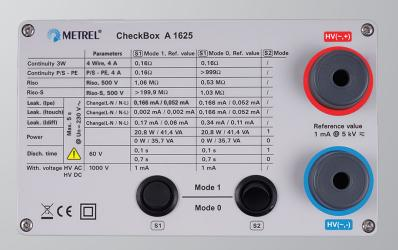
It is wise to regularly, on daily basis inspect the test system. CheckBox has a built in electronic components with reference values, which proof that the measuring system is operating correctly A 1625 CE checkbox is intended for checking of correct measurements for instruments like MI 3394, MI 3325, or with combination of mentioned one with A 1460, or with combination of mentioned one with A 1600 nlus one of connection hox.
