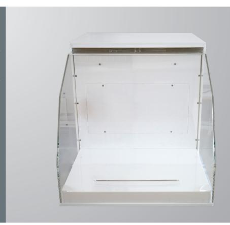
The A1650 Single chamber test cages provides automatic protection against direct contact. Its construction is designed "ready" for integration of RFID safety module. The safety module's "coded" RFID sensor is monitoring the "cage closed" position, this enables the test system to prevent touching of the DUT throughout the test sequence where dangerous voltages can occur. Passive tests can be normally generated also at opened doors. Malfunction or misuse is practically impossible
