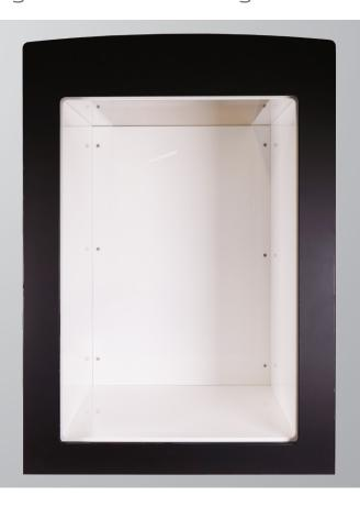
The A 1676 Single chamber test cage construction is designed "ready" for integration of light curtain safety module. The safety module provides the automatic protection against direct contact by light curtains. If the light curtain detects the bridge inside the prohibition zone, the safety module disconnects measuring circuits from the mains. No closing door is needed
