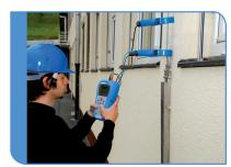
Two clamps method for testing ground resistance of object on TN system
