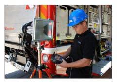
Testing of appliances locates faults in decreased insulation resistance because of dirt, dust, moisture.
