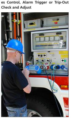
Applying an adjustable fault with the EurotestIM could prove the proper connection of Insulation Monitor protection Devices in the system and Alarm operating when currents exceeds the dangerous
