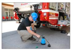
The purpose of this test is to ensure the proper operation of residual current devices (RCD) built into appliances / installations and portable residual current devices (PRCD). Trip-out time measurement verifies the sensitivity of a (P)RCD at selected residual currents.
