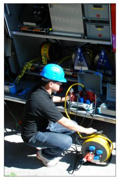
With the earth bond test all metal construction of the vehicle and the contacts between accessible metal parts on connected appliances are firm. Extension leads, IEC Leads, prolongation cords and Cables Polarity need to be checked. With the polarity test shorts, crossed and opened wires in cords can be found.
