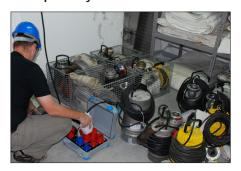
The purpose of this test is to ensure the proper operation of residual current devices (RCD) built into appliances / installations / extension leads and portable residual current devices (PRCD). Trip-out time measurement verifies the sensitivity of a (P)RCD at selected residual currents
