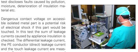
The purpose of this test is to ensure the proper operation of residual current devices (RCD) built into appliances / installations / extension leads and portable residual current devices (PRCD). Trip-out time measurement verifies the sensitivity
