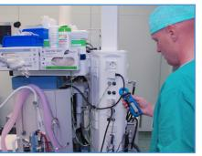
A simple method for localizing excessive leakage currents causing problems is the selective differential or direct Leakage / Fault Current measurement with current
