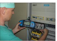
nsulation problem can be predicted in most cases before troubles arise when IMD monitors proper mounted and whether still operating. The EurotestIM makes it double checked by applying an adjustable fault and when currents exceeds the expected level it cause alarm indication of Insulation Monitoring Devices.
