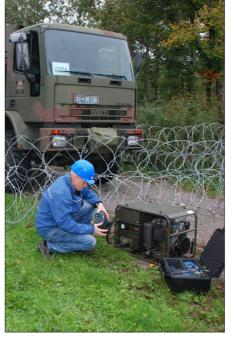
The EurotestIM applying an adjustable fault and when currents exceeds the expected level it cause alarm indication of monitoring devices. Insulation problem can be predicted in most cases before malfunction, operation fail, damages or IMD Insulation / ELM Earth Leakage / troubles arise when IMD monitors proper
