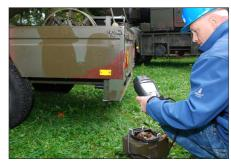
In this test the sum of leakage currents caused by appliance insulation is checked. The differential leakage current, the PE conductor (direct) leakage current and the touch leakage current are measured. Even leakage currents in range of mA are dangerous.
