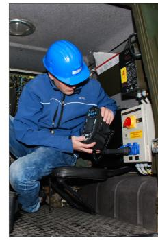
The EurotestIM makes automatic warnings on Voltage out of range to protect
