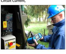
Limit barrieres are built-in the EurotestIM and the instrument generate warnings in case of improper protective devices are installed, bad connections, bad assembling, lenghts and cross section of wiring in installation and in case windings of generator / transformer are already damaged.
