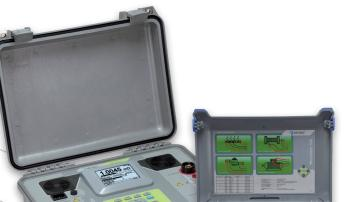
resistance and provide extremely accurate readings (0.25%). The instrument can be powered from mains supply or internal battery. PC SW HVLink PRO supplied as a standard accessory enables downloading, analysis and export of test results and printing of test
