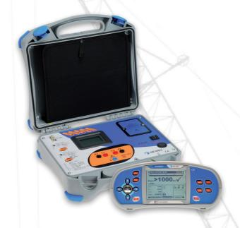
The A 1143 Euro Z 290 A is a professional portable high current impedance tester. It performs high precision line and fault loop impedance measurements in environments up to CAT IV / 300 V. It is used to test power transformers and motor windings. The main users are maintenance engineers in power utilities. The instrument is designed to work independently or in conjunction with the MI 2086 Eurotest 61557, MI 3101 EurotestAT, MI 3105 EurotestXA and MI 3321 MultiServicerXA.
