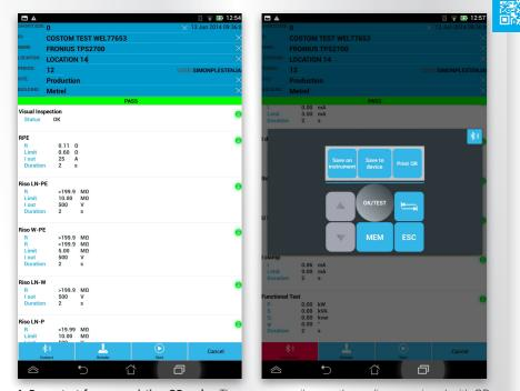
1. Run a test from an existing QR code: The user can easily scan the appliance equipped with QR code from previous testing containing information about previously performed test sequences, test results, limits and other user information. aPAT enables the user to simply repeat the test and print a new QR label, or store results to brand new or existing structure. This saves the user time and effort by not having to set up the sequences each time a retest is scheduled.
