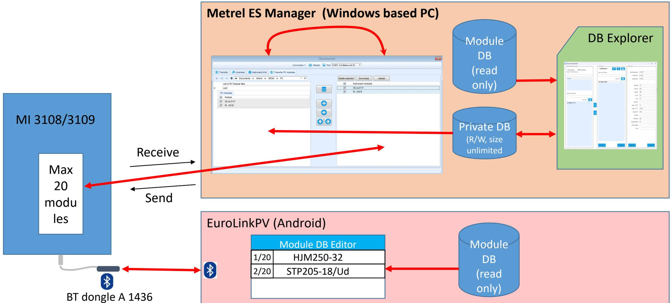
In PV Modules window you edit the 20 modules list – first Receive the existing list from instrument, then edit it (delete, change order or add from Private DB) and finally Send back to instrument.
