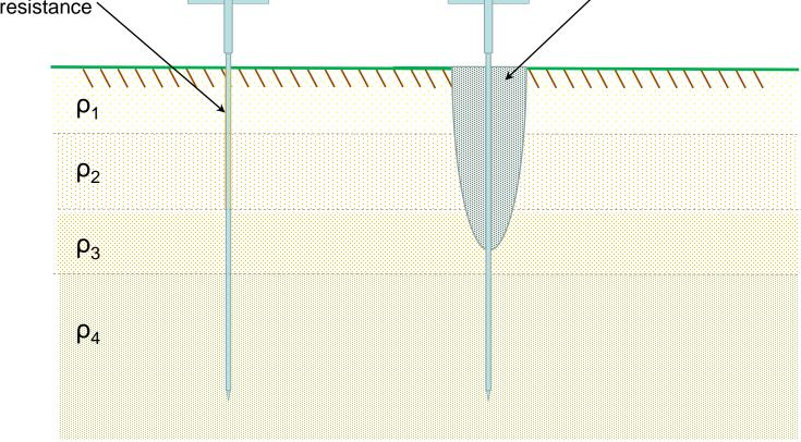
For step & touch voltage measurement the  $R_{C_{MAX}}$  is 275  $\Omega$  and if the minimum test current of 200mA can't be reached with one auxiliary probe, multiple probes connected in parallel have to be used .
