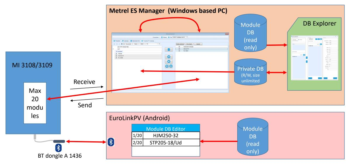
In PV Modules window you edit the 20 modules list – first Receive the existing list from instrument, then edit it (delete, change order or add from Private DB) and finally Send back to instrument.
